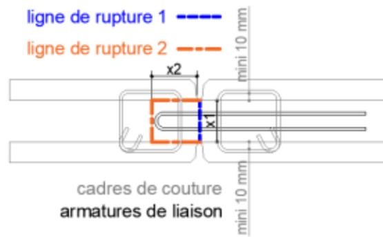
$$V_{Rd} = \min\{V_{Rd1}; V_{Rd2}\}$$
