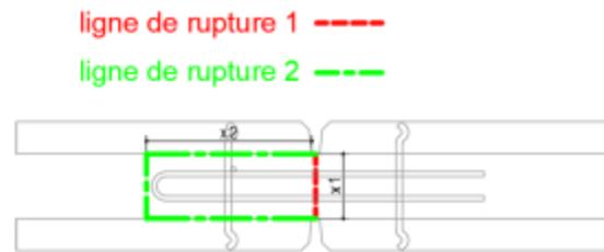
$$V_{Rd} = \min\{V_{Rd1}; V_{Rd2}\}$$
